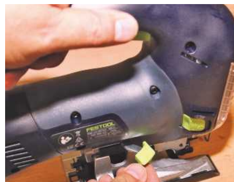
▲ This lever releases the clamps that hold the base in position
